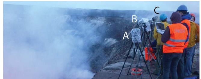
Fig. 3: Deployment of the cameras and related sensors on the rim of Kīlauea crater. The data from the camera are linked to information from the permanent recording networks of the Hawaiian Volcano Observatory giving a uniquely detailed record of explosions. Tripods house infrared (A), monochrome (B), and color (C) high speed cameras which are synchronized.
