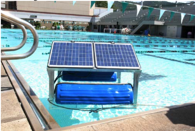
A newly constructed coastal gamma-spectrometer was constructed in collaboration with the SOEST Engineering Support Facility, shown here during its testing at UH. Dulaiova and Kamenik deployed the buoy in Heeia, Oahu in June 2013.
