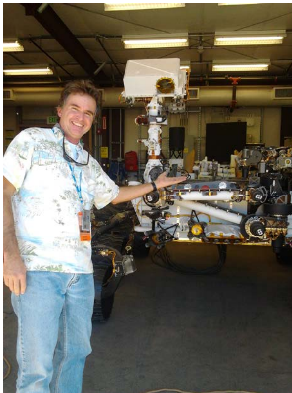
This is the testbed rover, an almost identical copy of Curiosity, which is used to practice potentially tricky maneuvers and to troubleshoot problems.
