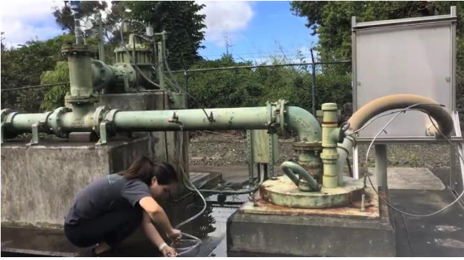
Brytne Okuhata setting up a copper tube and aluminum channel to sample groundwater for tritium/helium from a pumping well on the kona side of the Big Island.
