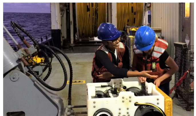
Graduate Students Charu Lata (UH) and Bridgit Boulahanis (Lamont) disassembling an ocean bottom seismometer.
